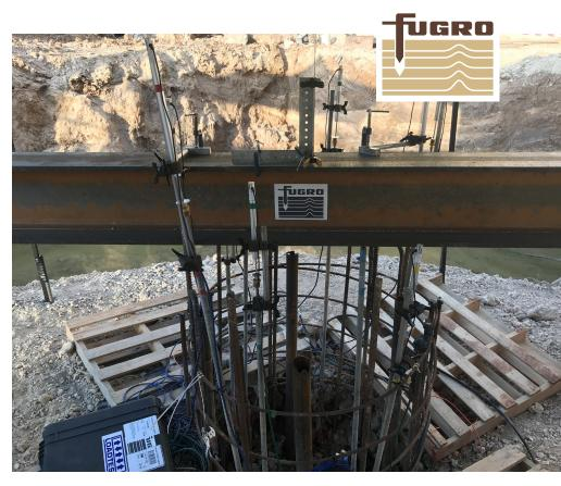
Testingunder way with reference beam system to determine pile head movements.
